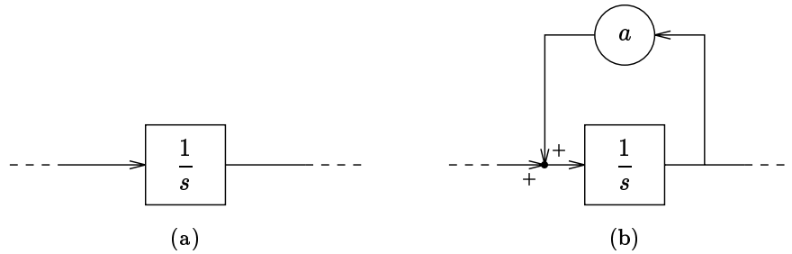
Figure 5.6 A realization of H(s - a) can be formed by taking each integrator in a realization of H(s) , shown in (a), and adding a feedback of a , as shown in (b).
